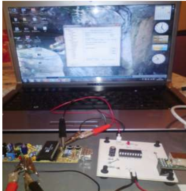
Figure 4.2(d): Complete hardware connections of the audio record/playback system
